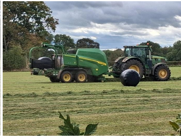
October the 5 th : The sweeper with round baler and showing the bale being wrapped in black plastic.
