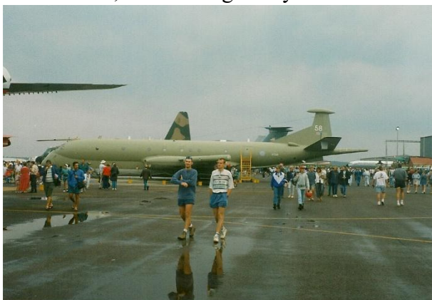
RAF BAe Nimrod Mk2. Notice the inflight refuelling probe and MAD tail boom.
