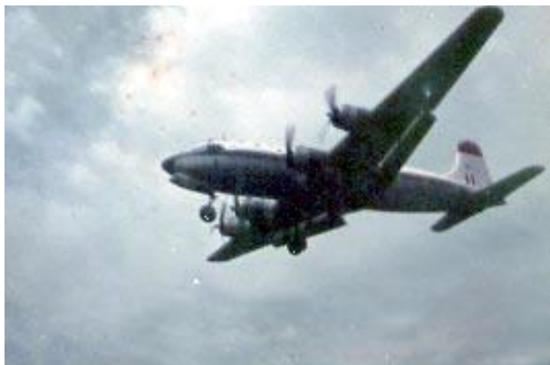
SAAF DC-4 on short finals with undercarriage down and flaps extended.
