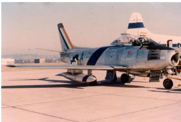
SAAF Sabre with under wing fuel tanks to increase range.
