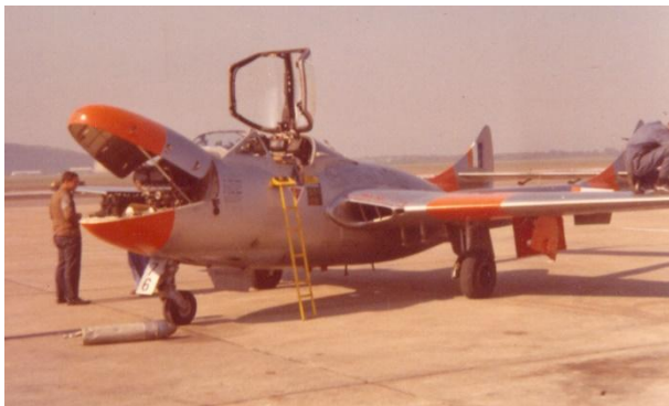
SAAF de Havilland Vampire T Mk55 in dayglo markings with nose equipment bay open and ground crew working on the wing.
