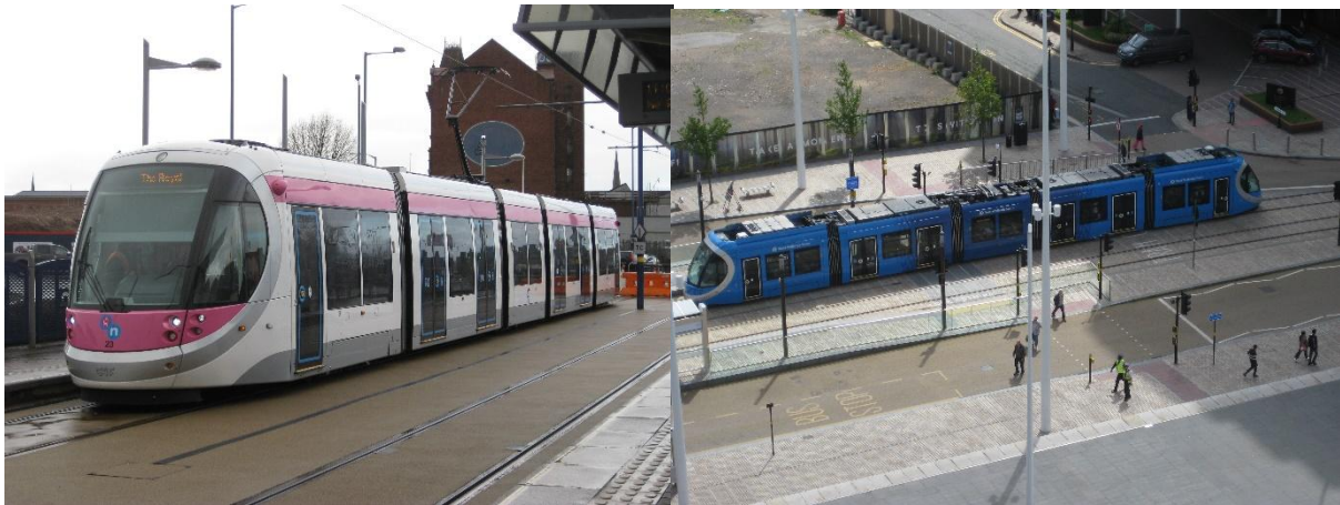
No. 23 at the then Royal terminus with the pantograph raised. No 56 (right) travelling with the pantographs stowed and no overhead cable network visible.
