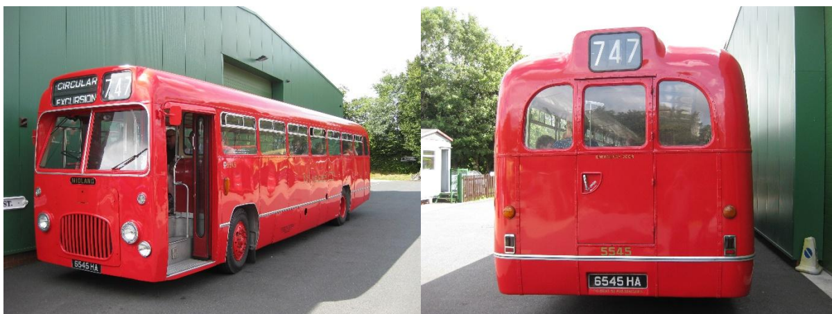
6545 HA showing the front door and rear emergency exit.
