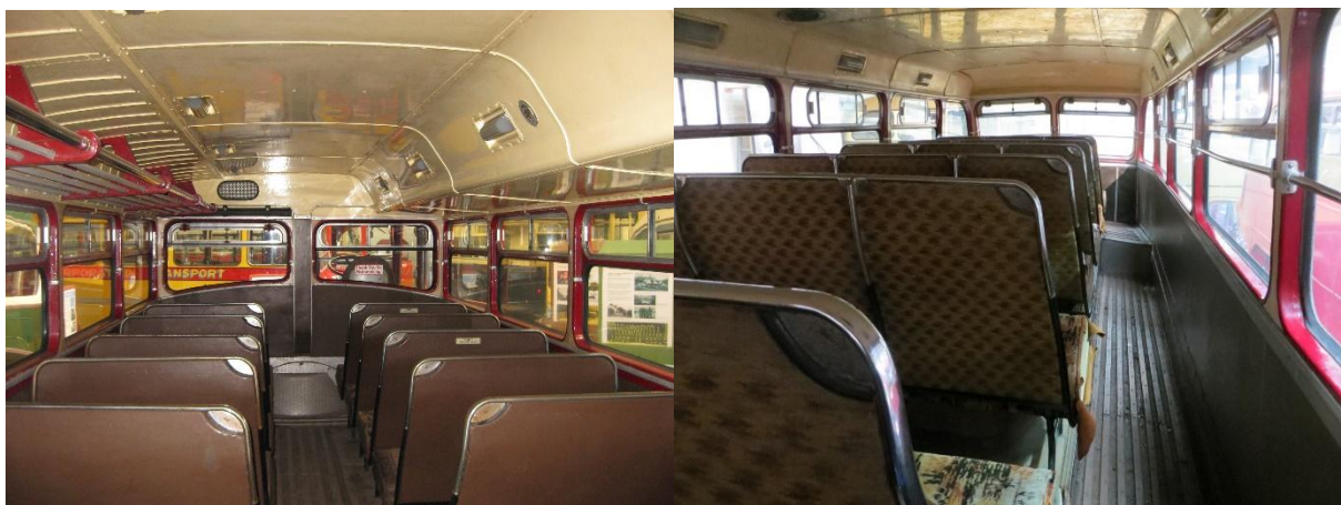
HWO 334. Lower deck right sunken ceiling and upper deck right lower gangway.
