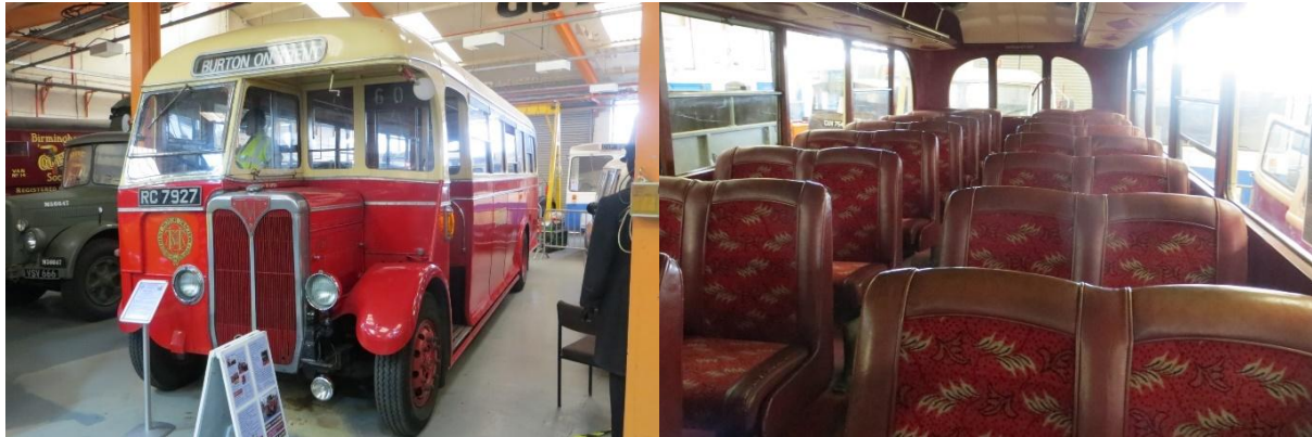
CVP 207. Left, half cab and front entrance. Right, well upholstered, rear emergency exit.
