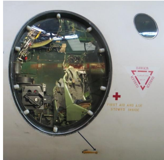
Photograph 2023-11-07. Emergency access Visible on the previous photograph) with external lever arrowed and showing the crew area.
