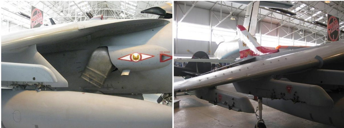
Photographs 2012-10-03. Notice the different nozzle compared with the Kestrel and two outer hard points on the right wing (repeated on the left wing).
