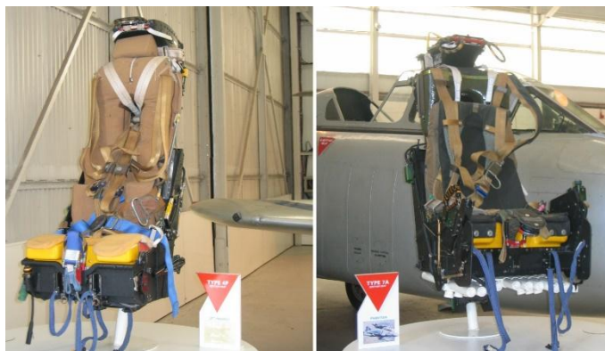
Photograph 2008-08-24. 4P and 7A ejection seats.
