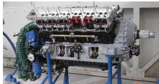
Photograph 2012-10-03. A Rolls-Royce Merlin 28 12 cylinder used in the Lancaster Mk.III and Curtiss Kittyhawk.
