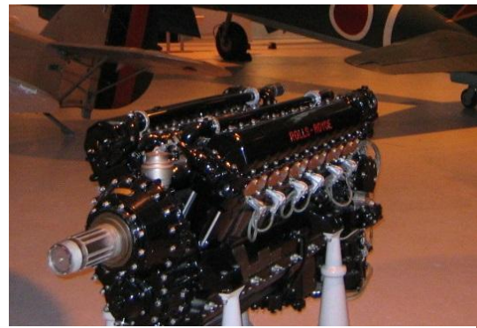
Photograph 2007-02-10. Rolls-Royce Kestrel XVI engine.
