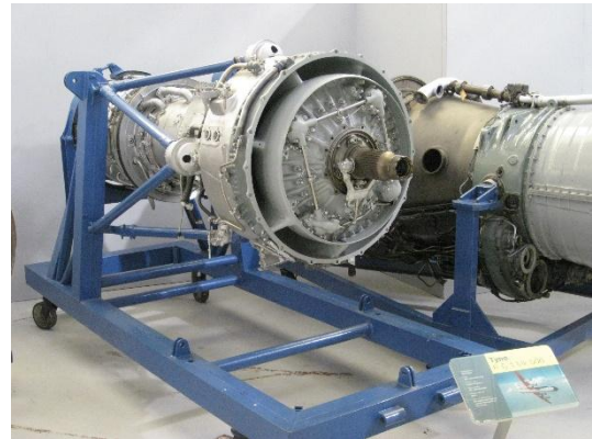
Photograph 2023-11-07. A Rolls-Royce Tyne RTy.1 Mk 506 turboprop.
