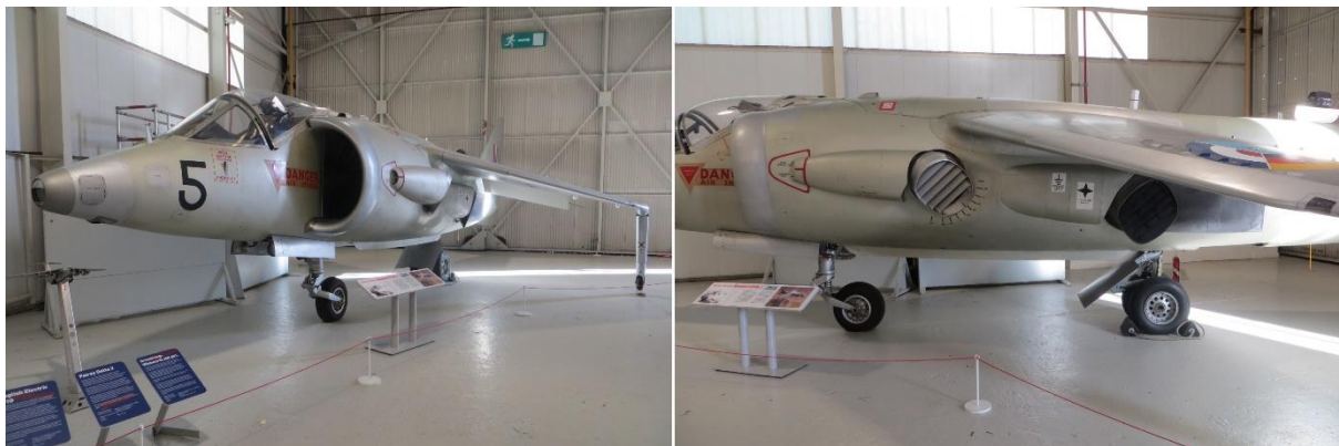
Photographs 2023-11-07. Adjustable nozzles seen on the right and tri-nation roundel.
