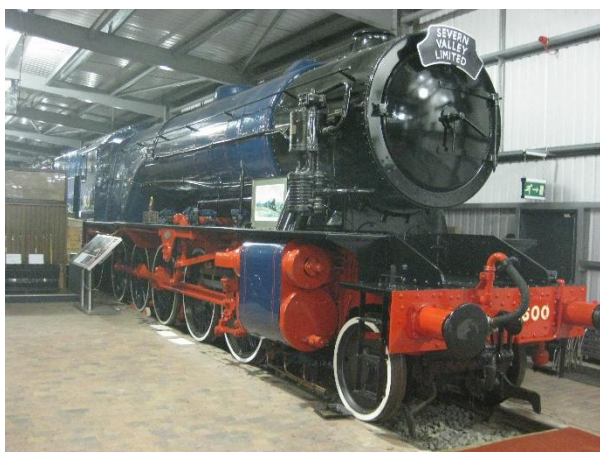
Left: Longmoor Military Railway (War Department) steam locomotive, number 600 Gordon, 2-10-0, 94 tons, designed by Riddles, built by North British Locomotives Co. in 1943. It is a World War II “Austerity” locomotive designed for freight operation.
