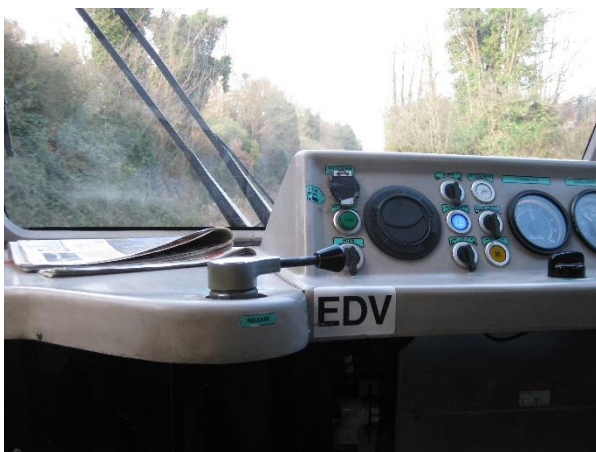
Left: the uphill track to Stourbridge Junction. Right: The controls of 139001. The handle is presumed to be the throttle. Behind the handle knob is the horn switch. Above it are the door controls. Right of the black disc (air vent?) is the saloon lights switch, below Cab/demist fan. Then top to bottom, screen wash, headlights and saloon heat. To the right is the flywheel RPM gauge next the vehicle speed MPH gauge.
