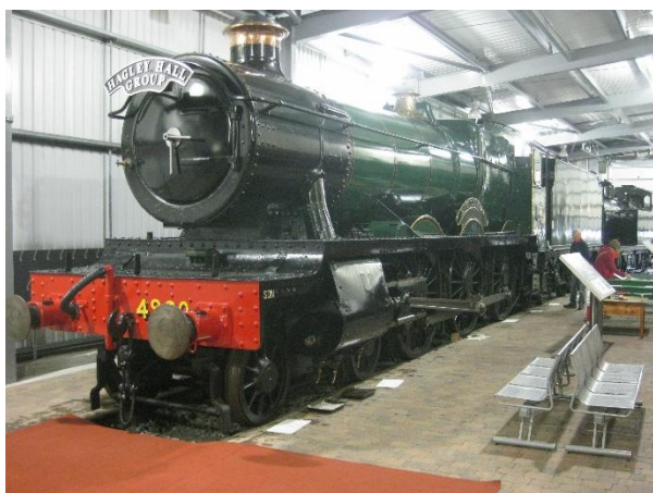
Above left: GWR steam locomotive, number 4930 Hagley Hall, Hall Class, 4-6-0, 121 tons. Designed by Collett, built at Swindon in 1929 (Williams, 2001). Above right: LMSR tank steam locomotive, number 47383, class 3F, 0-6-0T, 49 tons, designed by Fowler, built at Vulcan Foundry in 1926 (Williams, 2001).
