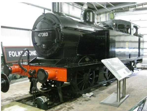
Above left: GWR steam locomotive, number 4930 Hagley Hall, Hall Class, 4-6-0, 121 tons. Designed by Collett, built at Swindon in 1929 (Williams, 2001). Above right: LMSR tank steam locomotive, number 47383, class 3F, 0-6-0T, 49 tons, designed by Fowler, built at Vulcan Foundry in 1926 (Williams, 2001).
